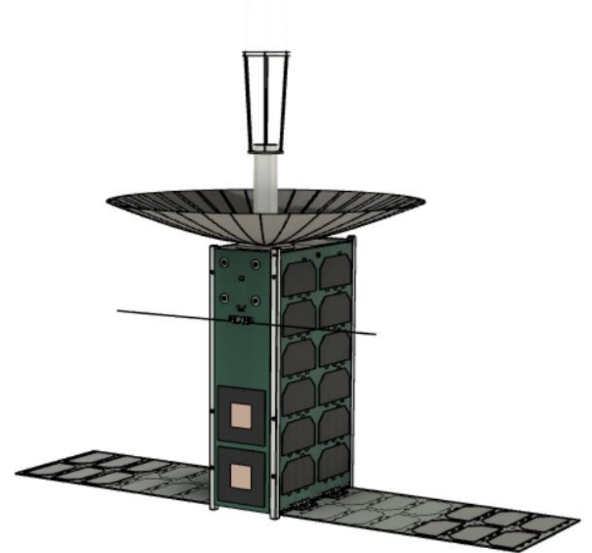
Figure 17: 6U CubeSat (Radar deployed)
