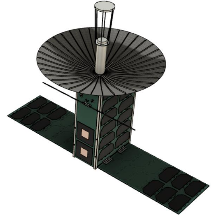
Figure 10: 6U CubeSat with radar CAD Model
